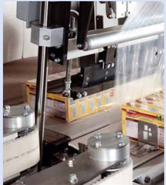
Siegling Proposition belts in a packaging machine.
