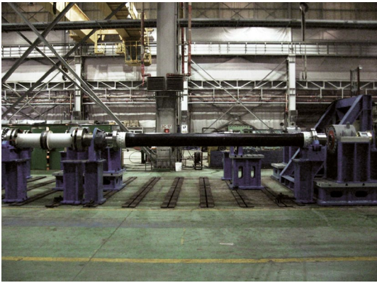
Lamidisc® coupling 605-8 with JCFS composite shafts
