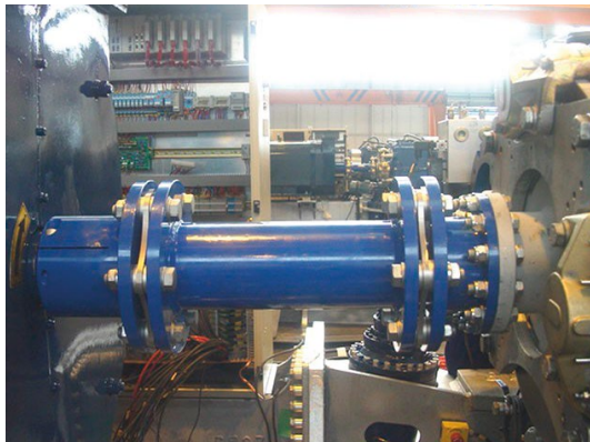
Lamidisc® coupling SXPR with adaptor flange
