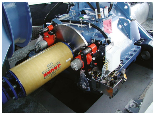
Lamidisc® coupling in combination with glass fiber shaft for electrical insulation
