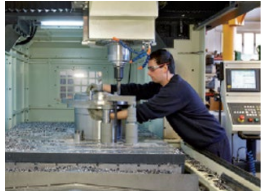
Machining of a barrel coupling hub
