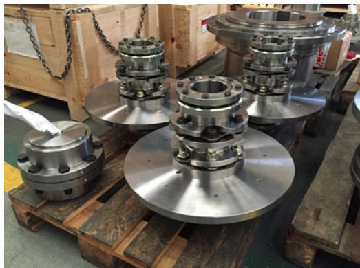
Disc pack configuration with brake disc.
