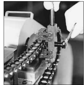
Fig. 5 How to cut a chain using a chain screw1 Rivet-type roller chain
