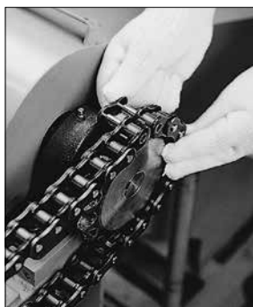
Fig. 8 Connecting on a sprocket
