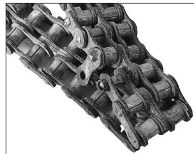
Fig. 34 Corrosion of stainless steel roller chain
