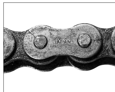
Fig. 35 Hydrogen embrittlement cracking
