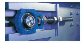
Screw tensioning device
