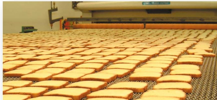
Balanced weave belt in furnace at Bolletje, Almelo, Holland.
