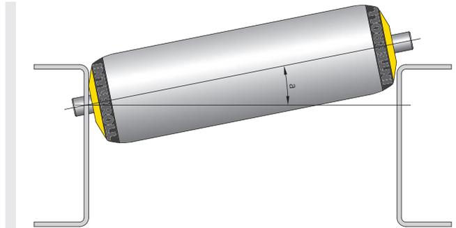
The following formula and the drawings should provide support in sufficiently dimensioning the fastening hole. For this purpose, an oversize of 0.5 mm of d1 compared to the shaft diameter is sufficient in most cases. In case of side profiles with different heights, the dimension H of the higher profile must always be used for the calculation.
