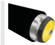
The PU sleeve ensures a high level of noise reduction, particularly for steel containers, and offers a high level of protection of sensitive conveying goods. An improved conveyance of conveying goods is achieved with the higher coefficient of friction compared with a steel tube. Conveying goods can easily be separated since the larger diameter leads to a higher speed with the same rotational speed. With mechanical stress, e.g. with abrasion, it offers a higher robustness than a PVC sleeve.
