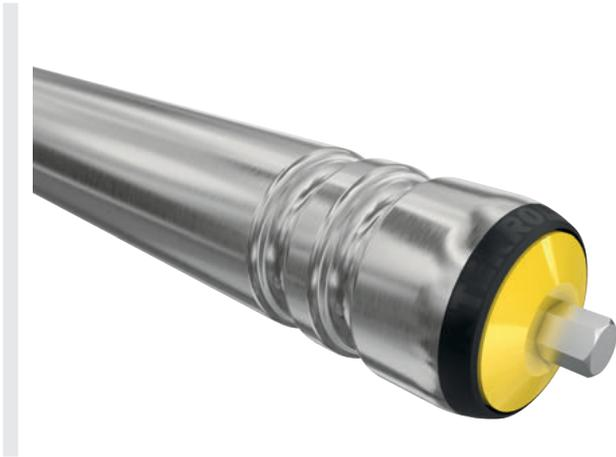
Grooves are running grooves that can be placed in steel tubes. They are used to guide round belts. When using the corresponding round belt, they are below the roller surface and, as such, do not contact the conveying good.
