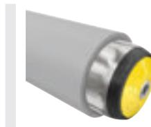
The PVC sleeve ensures a particularly high noise reduction and offers a high level of protection for sensitive conveying goods. An improved conveyance of conveying goods is achieved with the higher coefficient of friction compared with a steel tube. Conveying goods can easily be separated since the larger diameter leads to a higher speed with the same rotational speed.
