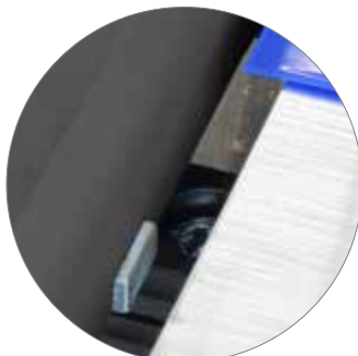
Insert bar for repeatable welds
