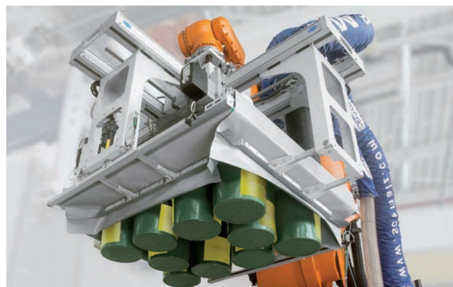
Vacuum layer gripping system SPZ handling buckets
