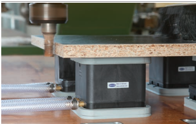
Vacuum block VCBL-G for gripping particle boards
