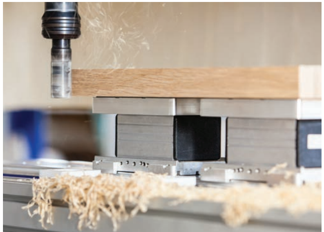
Vacuum block VCBL-K1 fixing a solid wooden board during CNC machining
