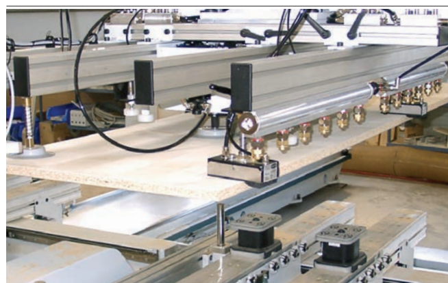
Area Gripping system FX-SW when handling wooden boards
