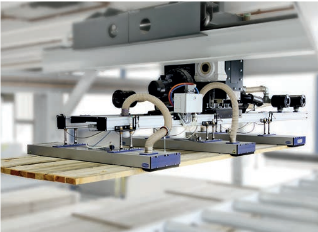
Suction spider SSP with area grippers SBX de-stacking wood in layers
