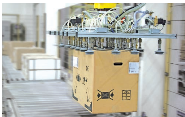
Bellows suction cups FSGA being used for handling cardboard boxes
