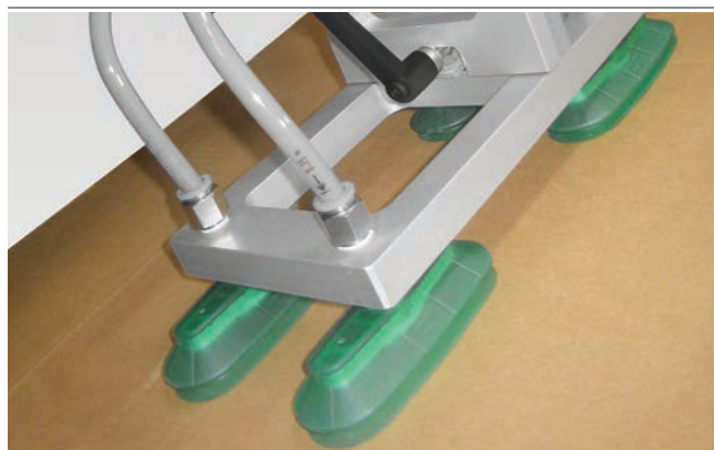
Bellows suction cups SPOB1 being used for handling of cardboard
