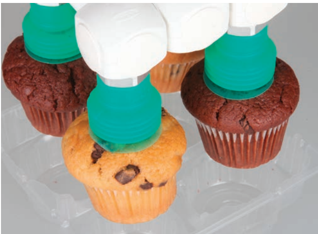
Vacuum suction cups SPB4f made from FDA-compliant silicone with vacuum end effectors VEE handling muffins
