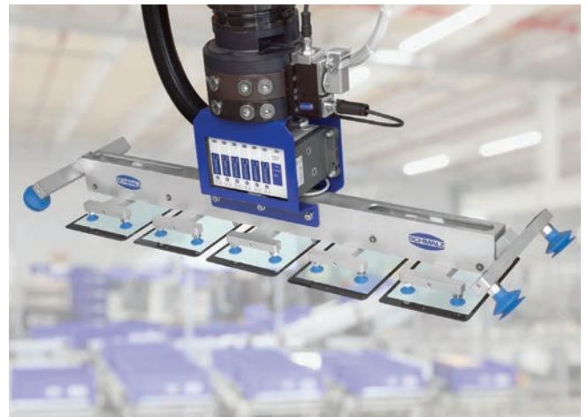
Vacuum suction cups FGA with a compact terminal SCTMi handling glass displays
