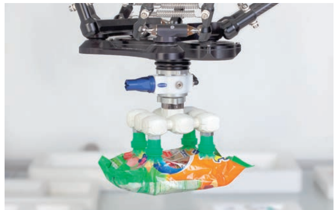
The vacuum end effector with bellows suction cups SPB4f handling pouches with strong wrinkling and low filling degree
