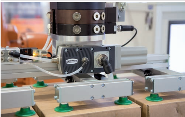
Centralized vacuum generation by means of basic ejectors SBPL
