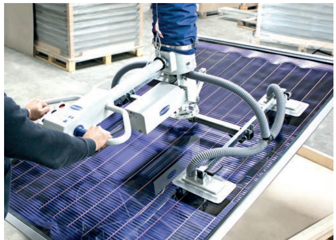
Tube lifter JumboErgo handling solar panels
