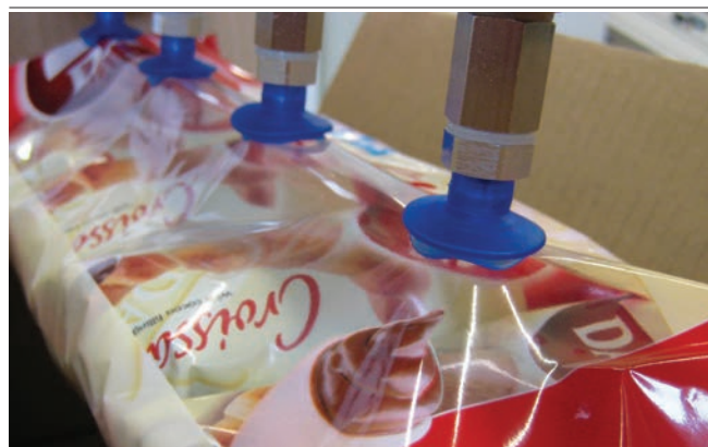
Bellows suction cups FGA PVC being used for handling non-rigid workpieces
