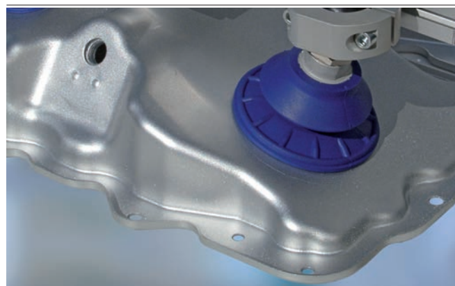
Bellows suction cups SAB being used for handling car bodywork parts
