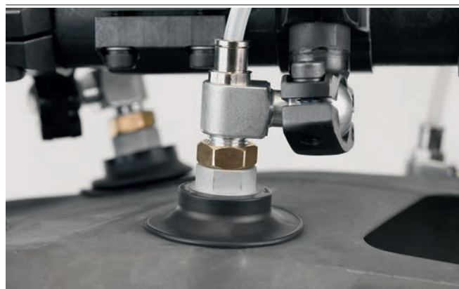
Flat suction cup SAF HT2 for handling formed sheet metal parts
