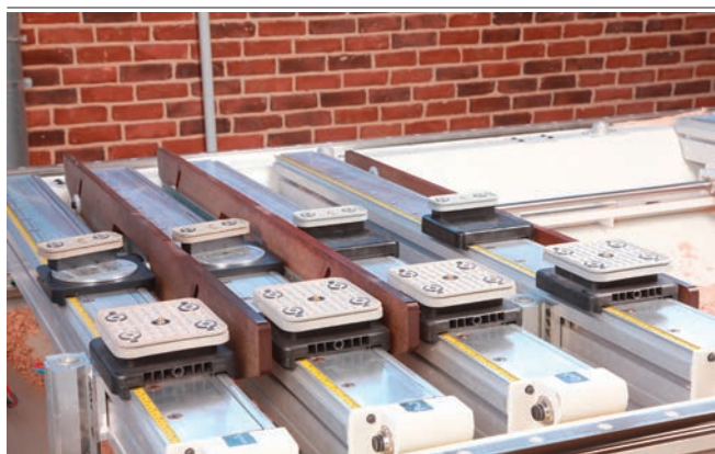
Vacuum block VCBL-S4 used with SCM consoles
