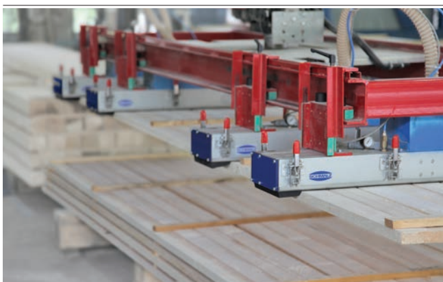
Area Gripping Systems SBX-C on an industrial gantry for handling unplanned wooden boards
