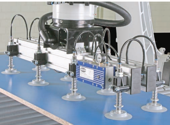
Vacuum suction cups SPC on a robotic spider loading a machine with coated wooden boards for furniture
