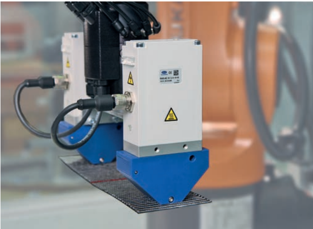
Needle gripper SNGi-AE handling composite textiles
