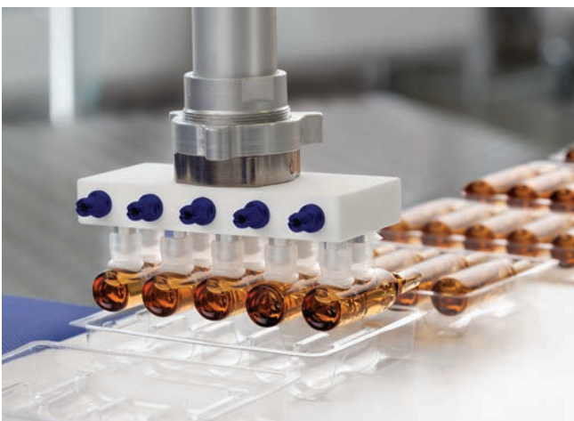
Gripper with vacuum suction cups made from FDA-compliant silicone and with integrated vacuum generation handling ampoules
