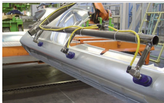
Bellows suction cups SAOB being used for handling car bodywork components
