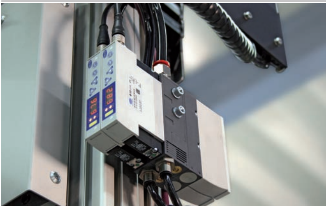
Centralized vacuum generation by compact ejectors SMPi
