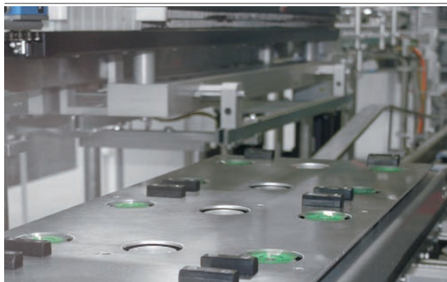
Flat suction cups SPF for use in carton erectors
