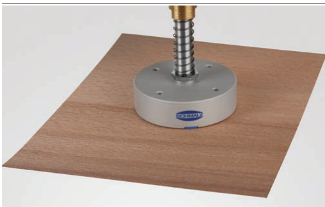
Floating suction cups SBS being used for handling thin wood veneer
