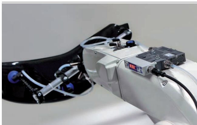
Centralized vacuum generation by means of compact ejector SCPSi
