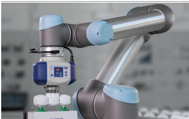
Electric vacuum generator ECBPi when handling cardboard boxes
