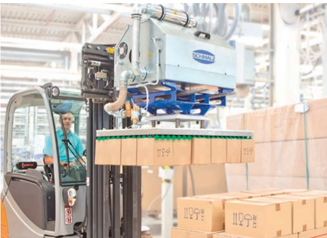
Layer gripping system SPZ order picking cardboard boxes on a forklift
