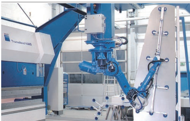
Flat suction cups SAF being used for handling sheet metal parts
