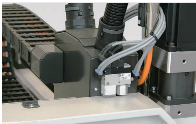
Central vacuum generation by compact ejectors SCPM
