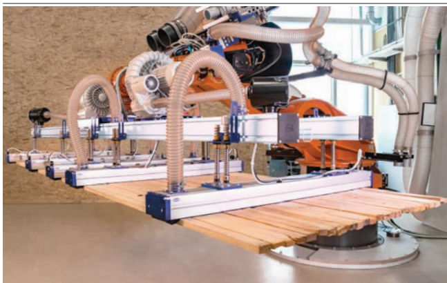
Area Gripping system FMHD handling rough sawn wooden boards
