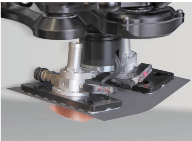
Schmalz area grippers for the dynamic handling of electrodes
