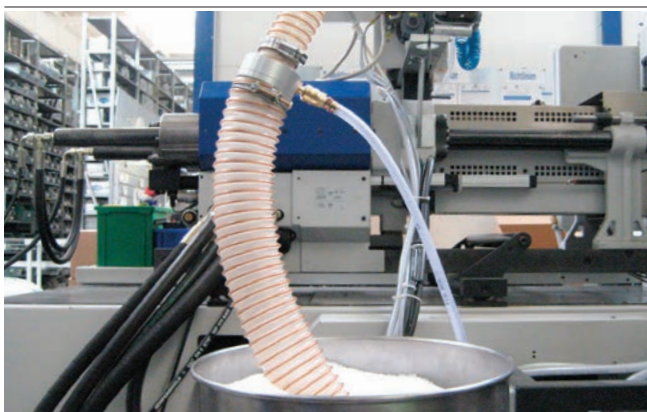
Feed Ejector SEC for transporting granulates
