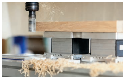
Securely clamp both flat workpieces and three-dimensional free-form surfaces.
