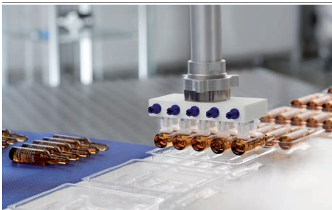
Vacuum generation by ejector modules SEP for handling ampoules
