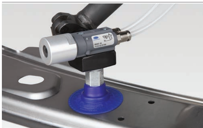
Decentral vacuum generation by ejector SEAC directly at the suction cup
