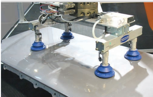
Suction cups with inline valves IV being used for handling carbody parts
