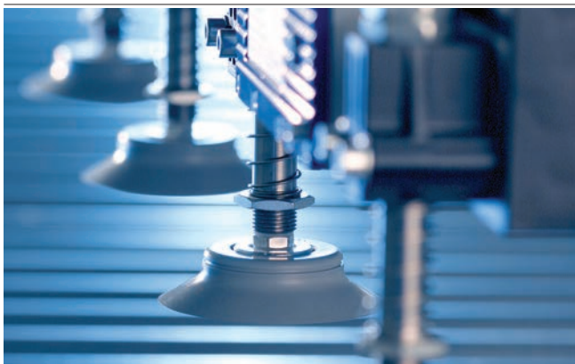
Suction plates SPU being used for handling shaped sheet metal parts
