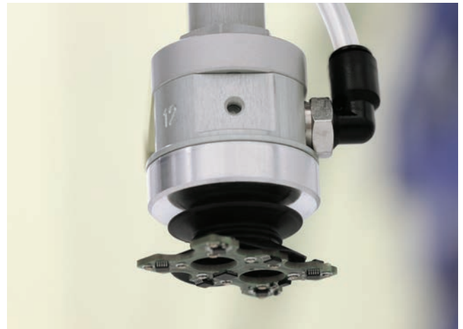
Flow grippers SCG handling assembled printed circuit boards
