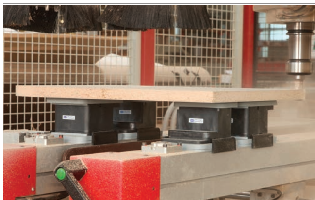
Vacuum block VCBL-K2 while clamping a workpiece
