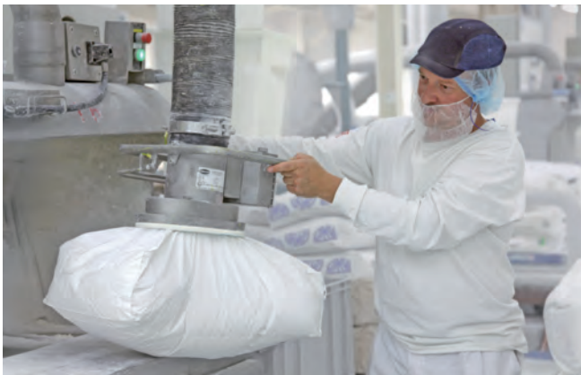
Vacuum tube lifter JumboSprint Ex for handling paper bags in an explosion protection zone
