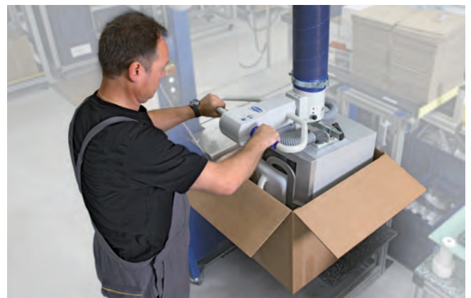
Vacuum tube lifter JumboErgo for packaging goods into boxes and handling the sealed boxes
