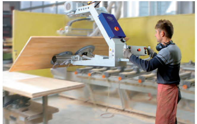
Vacuum lifting device VacuMaster Comfort for turning coated wooden boards by 180°
