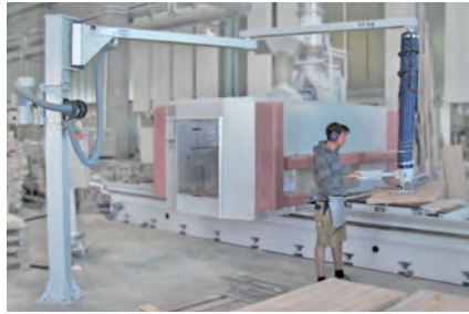
Articulated-arm jib to move around obstacles
