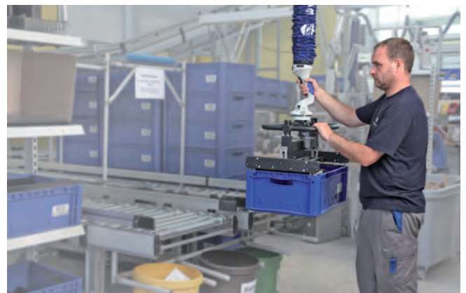
Custom solutions | Vacuum tube lifter JumboFlex for handling transport and storage boxes
