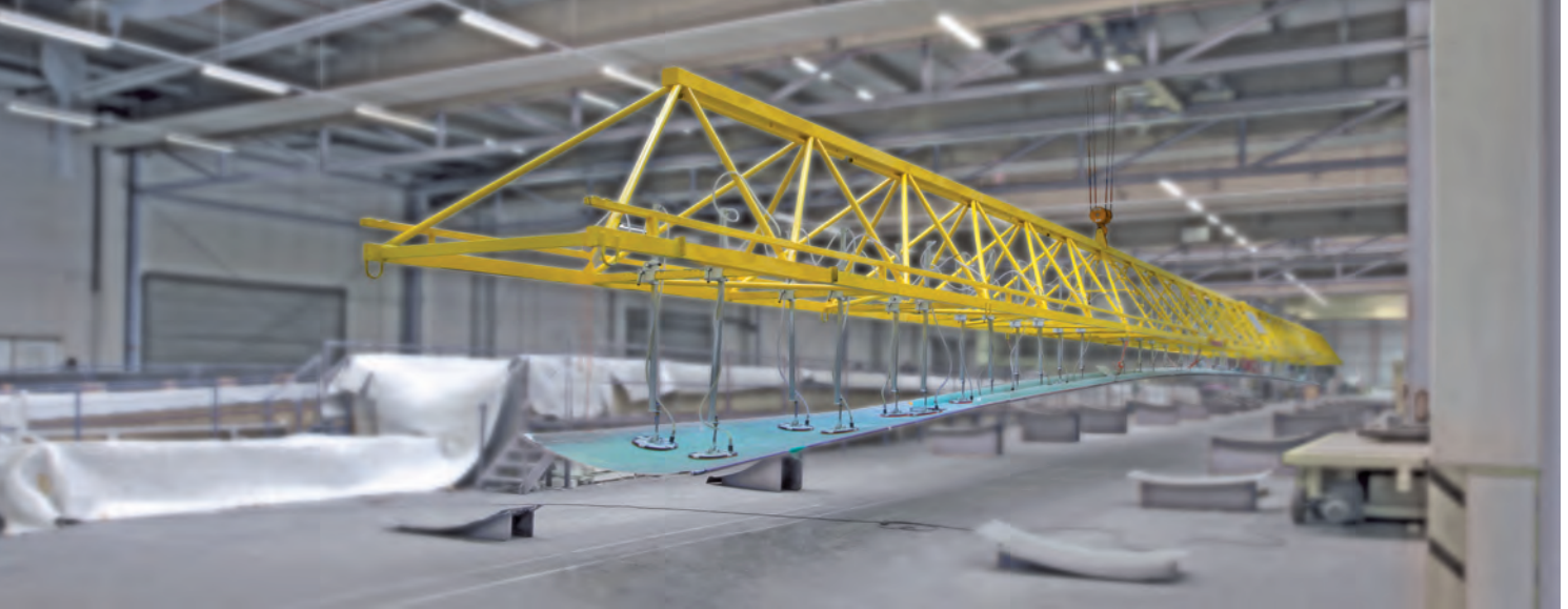
Wind energy | Vacuum lifting device VacuMaster for GRP components in rotor blade manufacturing weighing several tons and up to 60 m in length
