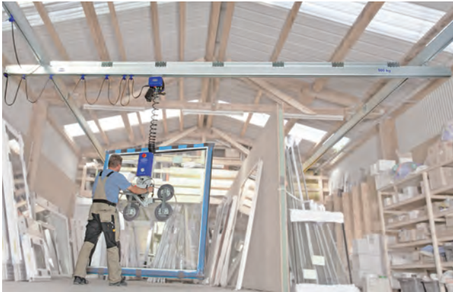
Aluminum crane system SRA with a chain hoist and vacuum lifting device VacuMaster
