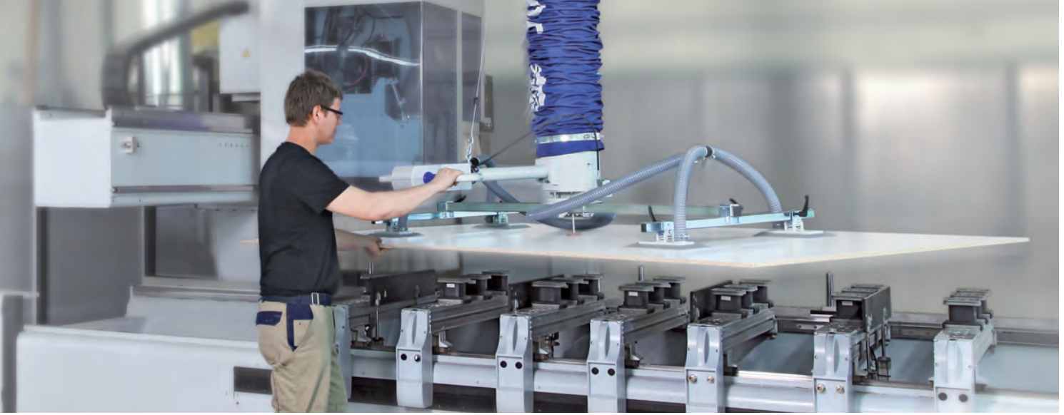
Vacuum tube lifter JumboErgo for loading and unloading a CNC machining center
