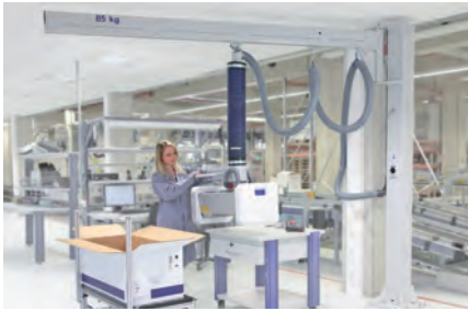
Flat jib for particularly low ceilings
