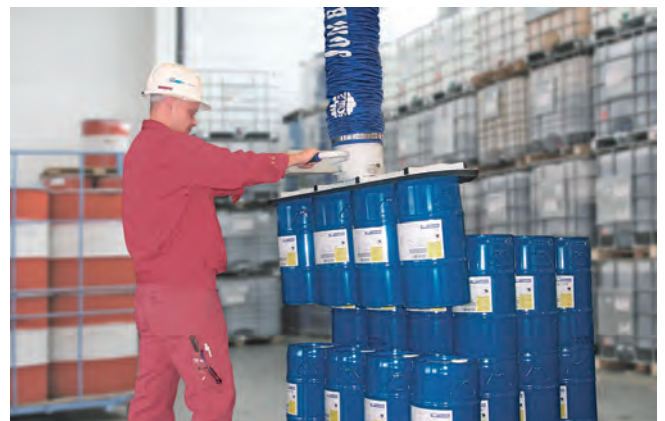
Vacuum tube lifter JumboErgo with large-area gripper for handling four barrels at once
