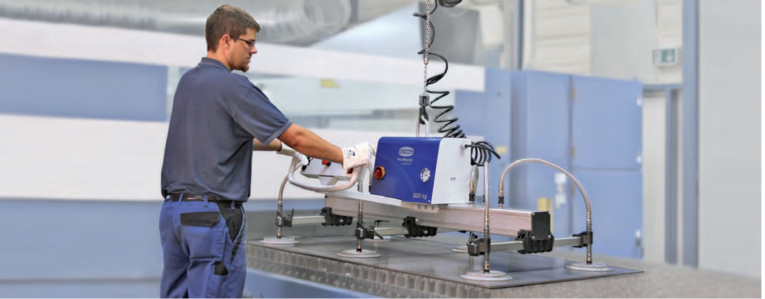
Vacuum lifting device VacuMaster Comfort for loading and unloading a laser cutting machine
