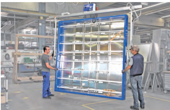
Custom solutions | Vacuum lifting device VacuMaster Box employed in the assembly of large advertising signs
