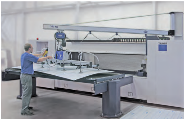
The TRUMPF TruLaser 1030 integrated loading solution: consists of vacuum lifting device VacuMaster Basic and column-mounted jib crane
