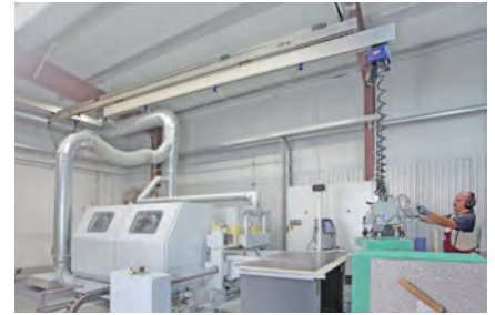
Telescopic jib for confined working areas
