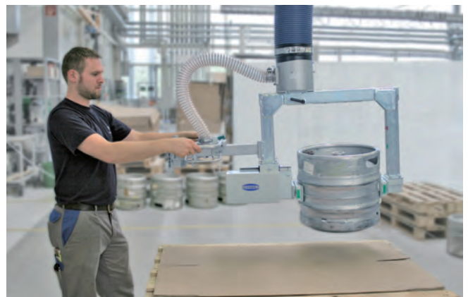
Beverage industry | Vacuum tube lifter JumboErgo with mechanical pneumatic grippers for lifting and turning kegs
