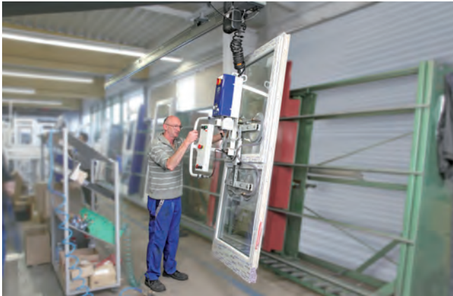
Vacuum lifting device VacuMaster Window Comfort for vertical handling of a multi-sash window
