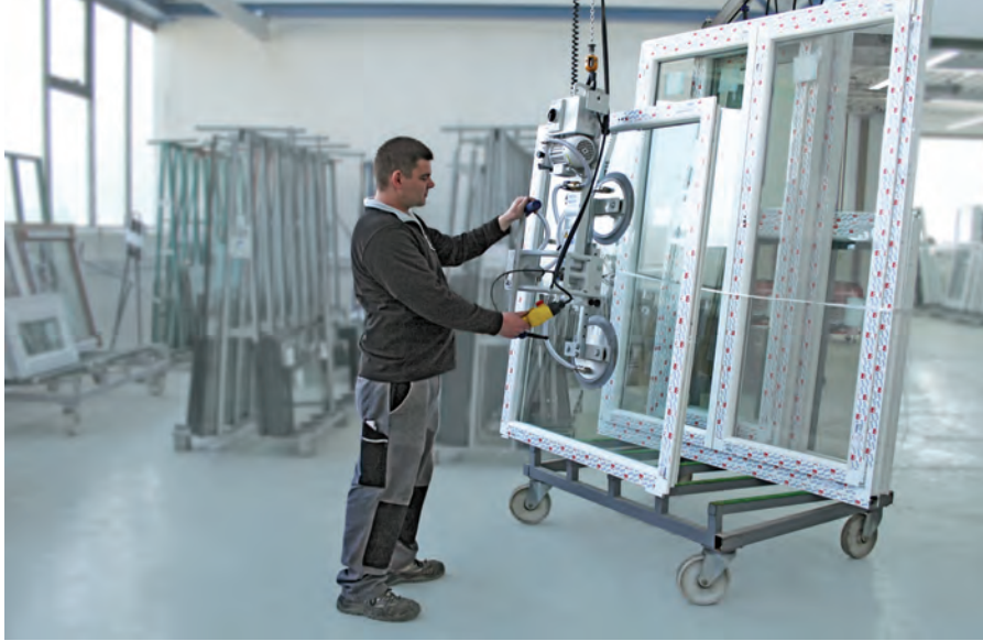
VacuMaster Window for rotating and palletizing windows
