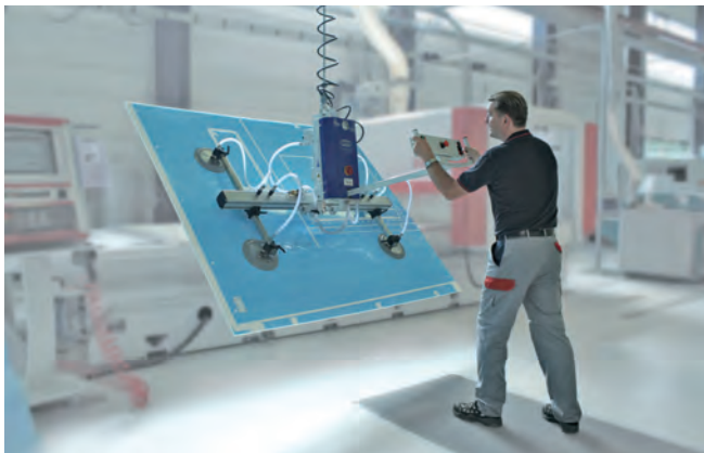
Plastics | Vacuum lifting device VacuMaster Comfort with 90° swivel angle for handling plastic sheets
