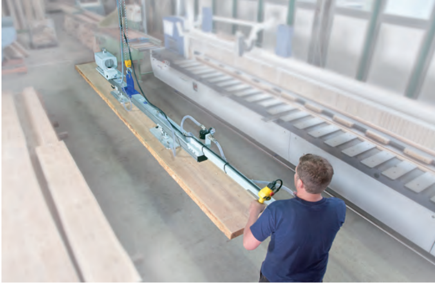
VacuMaster VHB in process of loading a rip saw with wooden boards
