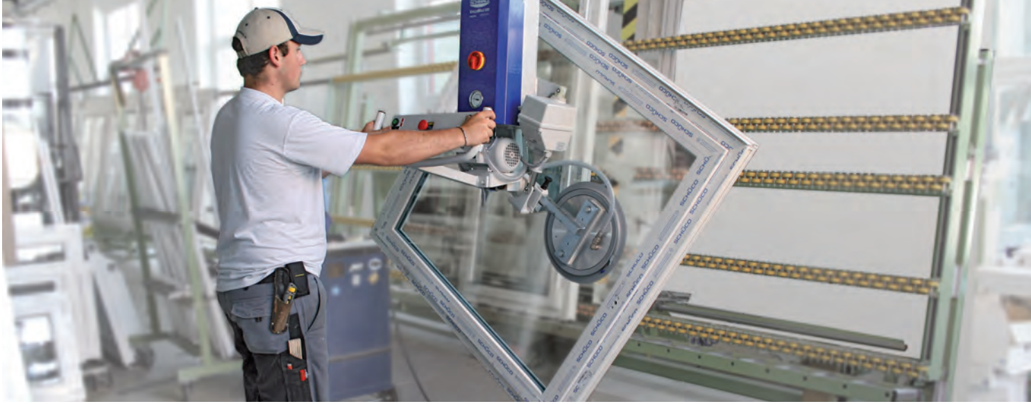
Vacuum lifting device VacuMaster Window Comfort for loading and unloading a glazing press
