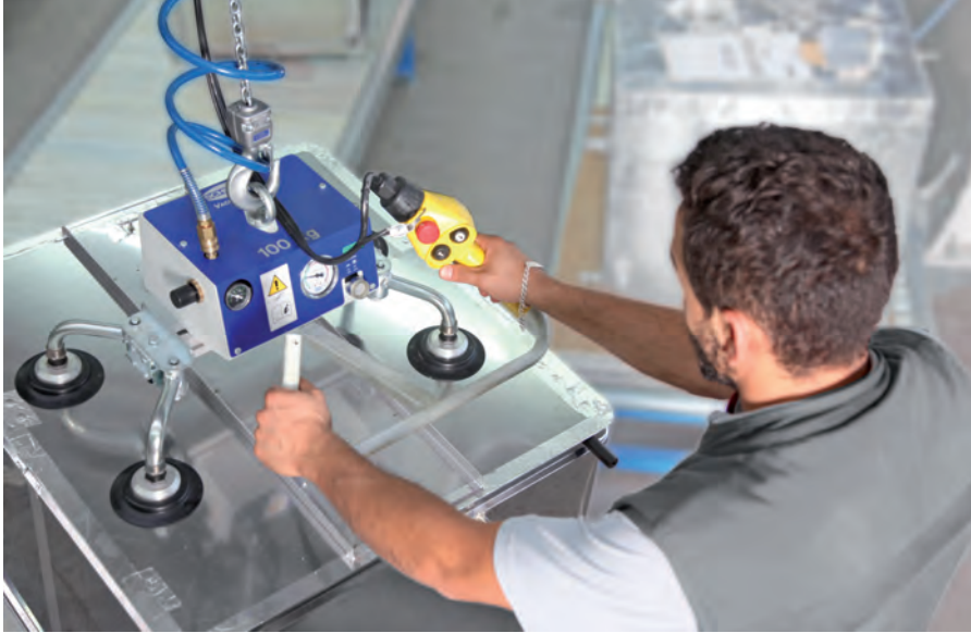
VacuMaster Light for handling metal housings
