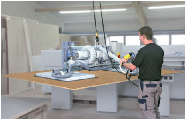
Vacuum lifting device VacuMaster Multi with 90° swivel angle for handling heavy, porous wooden boards
