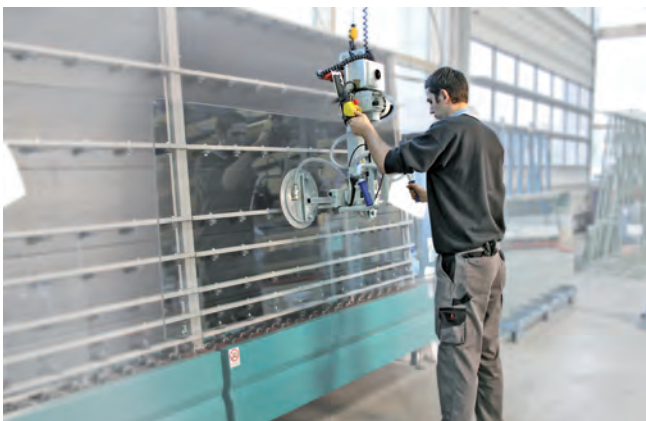
Vacuum lifting device VacuMaster Window for vertical handling of a glass sheet in a washing system
