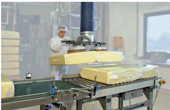
Food industry | Vacuum tube lifter JumboErgo for handling blocks of cheese
