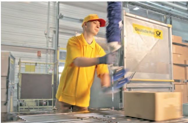
Vacuum tube lifter JumboFlex for lifting packages and for loading sorting and distribution machines
