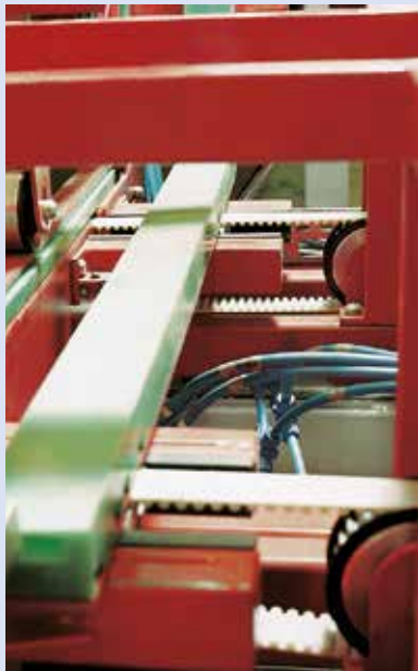
Conveying of car windows by belts running synchronously. The coverings on the reverse face of the timing belts treat the goods gently and improve the grip.
