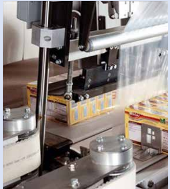
Siegling Proposition belts in a packaging machine.
